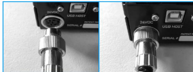
**IMPORTANT:** Always ensure that the Power Connector is fastened snugly into the Power Input of the PATCH System Hardware.
